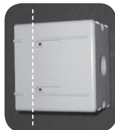
Slider plate in full forward position sets box for 1/2" drywall.
