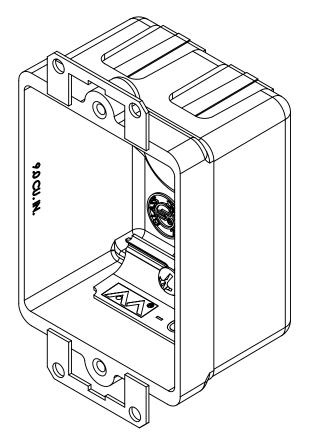
1.) BOX MATERIAL: FIBERGLASS REINFORCED POLYESTER, EAR MATERIAL: GALVANIZED STEEL, WIRE CLAMP MATERIAL: GALVANIZED STEEL, WIRE CLAMP SCREW MATERIAL: ZINC PLATED STEEL 2.) UL LISTED WITH 2 HOUR FIRE RATING FOR
