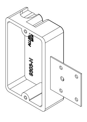
NOTES: 1.) BOX MATERIAL: FIBERGLASS REINFORCED POLYESTER, MOUNTING BRACKET MATERIAL: GALVANIZED STEEL
