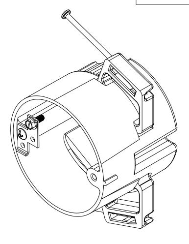
1.) BOX MATERIAL: FIBERGLASS REINFORCED POLYESTER, NAIL MATERIAL: PLATED CARBON STEEL, GROUND STRAP MATERIAL: GALVANIZED STEEL, GROUND STRAP MOUNTING SCREW MATERIAL: ZINC PLATED STEEL, GROUND SCREW MATERIAL: GREEN ZINC PLATED STEEL, SPEED KLAMP MATERIAL: PVC
