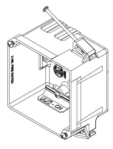
1.) BOX MATERIAL: FIBERGLASS REINFORCED POLYESTER, NAIL MATERIAL: PLATED CARBON STEEL, SCREW MATERIAL: ZINC PLATED STEEL, WIRE CLAMP MATERIAL: GALVANIZED STEEL, WIRE CLAMP SCREW MATERIAL: ZINC PLATED STEEL
