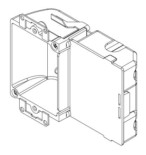
NOTES: 1.) BOX MATERIAL: FIBERGLASS REINFORCED POLYESTER, WING MATERIAL: GALVANIZED STEEL, WING SCREW MATERIAL: ZINC COATED STEEL, EAR MATERIAL: GALVANIZED STEEL
