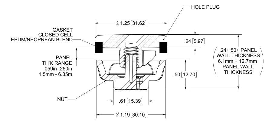
PLUGGED HOLE DIA RANGE: .812in-.937in 20.62mm-23.80mm
