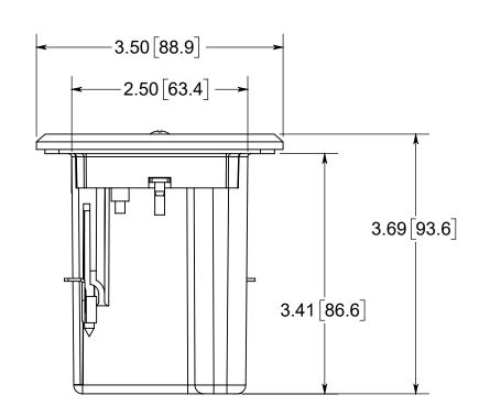
1.) BOX MATERIAL: POLYCARBONATE, COVER PLATE MATERIAL: BRASS, COVER PLATE MOUNTING SCREW MATERIALS: BRASS, DEVICE MOUNTING SCREW MATERIALS: ZINC PLATED STEEL, FLANGE MOUNTING SCREW MATERIALS: BLACK PHOSPHATE COATED STEEL WING MATERIAL: ZINC PLATED STEEL, GROUND PLATE MATERIAL: ZINC PLATED STEEL, GASKET MATERIAL: SINC PLATED STEEL, GASKET MATERIALS: POLYURETHANE FOAM 2.) UL LISTED, FLOOR BOX MEETS UL514C SCRUB WATER EXCLUSION TEST
