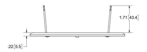
NOTES: 1.) COVER PLATE MATERIAL: DARK BRONZE PLATED BRASS, COVER PLATE MOUNTING SCREW MATERIAL: DARK BRONZE PLATED BRASS, GASKET MATERIALS: POLYURETHANE FOAM, O-RING MATERIAL: 2.) WHEN USED WITH FB-5DB FLOOR BOX IT IS UL LISTED, FLOOR BOX MEETS UL514C SCRUB WATER EXCLUSION TEST
