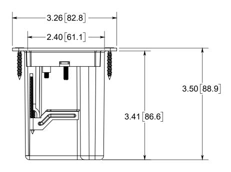
1.) BOX MATERIAL: POLYCARBONATE, DEVICE MOUNTING SCREW MATERIALS: ZINC PLATED STEEL, FLANGE MOUNTING SCREW MATERIALS: BLACK PHOSPHATE COATED STEEL WING MATERIAL: ZINC PLATED STEEL, GROUND PLATE MATERIAL: ZINC PLATED STEEL,
