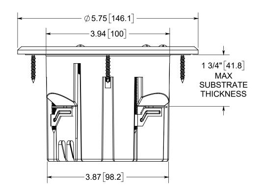
1.) BOX MATERIAL: POLYCARBONATE, COVER PLATE MATERIAL: DARK BRONZE PLATED BRASS, COVER PLATE MOUNTING SCREW MATERIAL: DARK BRONZE PLATED BRASS, DEVICE SCREW MATERIALS: ZINC PLATED STEEL, FLANGE MOUNTING SCREW MATERIAL: BLACK PHOSPHATE COATED STEEL WING MATERIAL: ZINC PLATED STEEL, GROUND PLATE MATERIAL: ZINC PLATED STEEL, GASKET MATERIALS: POLYURETHANE FOAM, O-RING MATERIAL:
