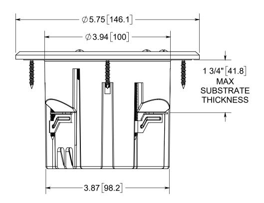
NOTES: 1.) BOX MATERIAL: POLYCARBONATE, COVER PLATE MATERIAL: NICKLE PLATED BRASS, COVER PLATE MATERIAL. NICKLE PLATED BRASS, COVER PLATE MOUNTING SCREW MATERIALS: NICKLE PLATED BRASS, DEVICE SCREW MATERIALS: ZINC PLATED STEEL, FLANGE MOUNTING SCREW MATERIAL: BLACK PHOSPHATE COATED STEEL WING MATERIAL: ZINC PLATED STEEL, GROUND PLATE MATERIAL: ZINC PLATED STEEL, GASKET MATERIALS: POLYURETHANE FOAM, O-RING MATERIAL: SILICONE 2.) UL LISTED, FLOOR BOX MEETS UL514C SCRUB WATER EXCLUSION TEST
