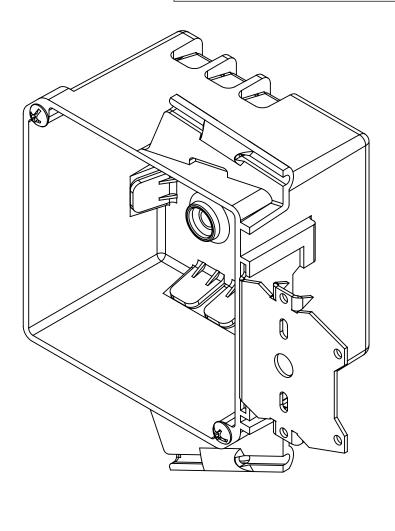
NOTES: 1.) BOX MATERIAL:POLYCARBONATE, MOUNTING BRACKET MATERIAL: GALVANIZED STEEL, SCREW MATERIAL: ZINC PLATED STEEL 2.) UL LISTED WITH 2 HOUR FIRE RATING FOR WALL
