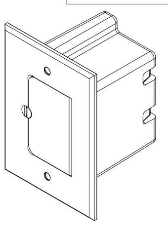
1.) BOX MATERIAL: POLYCARBONATE, BOX PLATE MATERIAL: POLYCARBONATE, PLATE MATERIAL: DARK BRONZE PLATED BRASS, COVER PLATE MOUNTING SCREW MATERIALS: DARK BRONZE PLATED BRASS, DEVICE MOUNTING SCREW MATERIALS: ZINC PLATED STEEL, FLANGE MOUNTING SCREW MATERIALS: BLACK PHOSPHATE COATED STEEL WING MATERIAL: ZINC PLATED STEEL, GROUND PLATE MATERIAL: ZINC PLATED STEEL, GASKET MATERIALS: POLYURETHANE FOAM 2.) UL LISTED, FLOOR BOX MEETS UL514C SCRUB WATER EXCLUSION TEST
