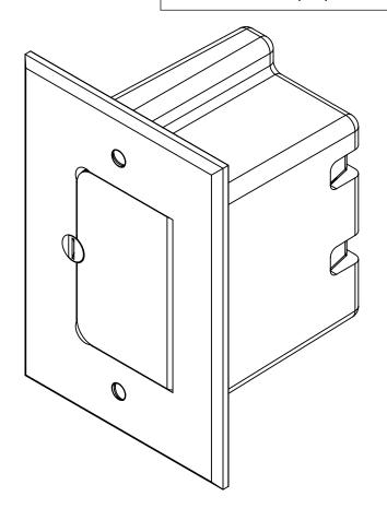
1.) BOX MATERIAL: POLYCARBONATE, BOX PLATE MATERIAL: POLYCARBONATE, PLATE MATERIAL: NICKLE PLATED BRASS, COVER MOUNTING SCREW MATERIALS: NICKLE PLATED BRASS, DEVICE MOUNTING SCREW MATERIALS: ZINC PLATED STEEL, FLANGE MOUNTING SCREW MATERIALS: BLACK PHOSPHATE COATED STEEL WING MATERIAL: ZINC PLATED STEEL, GROUND PLATE MATERIAL: ZINC PLATED STEEL, GASKET MATERIALS: POLYURETHANE FOAM
